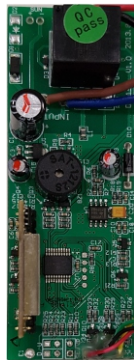
AVA-350A RF Receiver (For 24 Vdc Motor)
